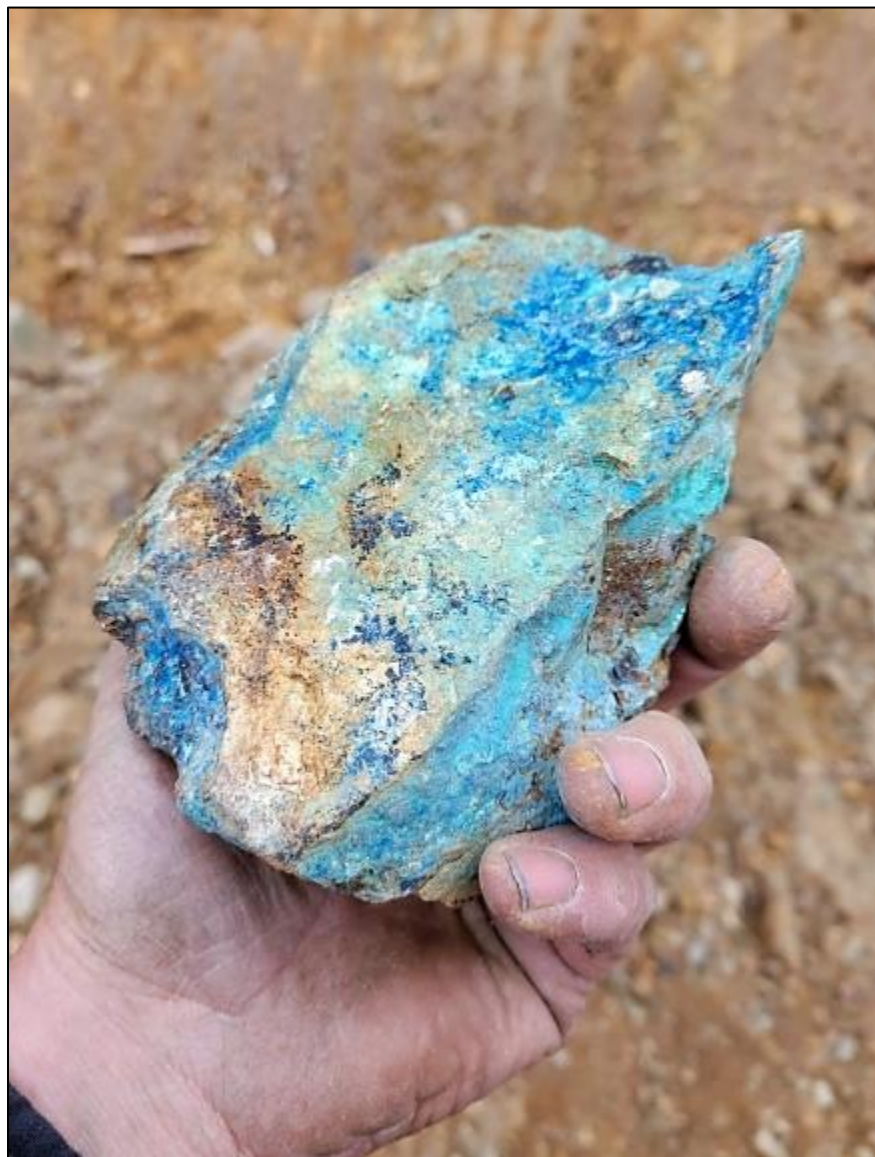
Figure 4: Grab sample from untested Blue target area, central MPD property. Altered diorite porphyry with azurite-malachite-chalcopyrite. Sample is from a 0.3 metre wide sample assaying 3.19% Cu, 0.21 g/t Au and 40.5 g/t Ag reported in news release February 3, 2022
